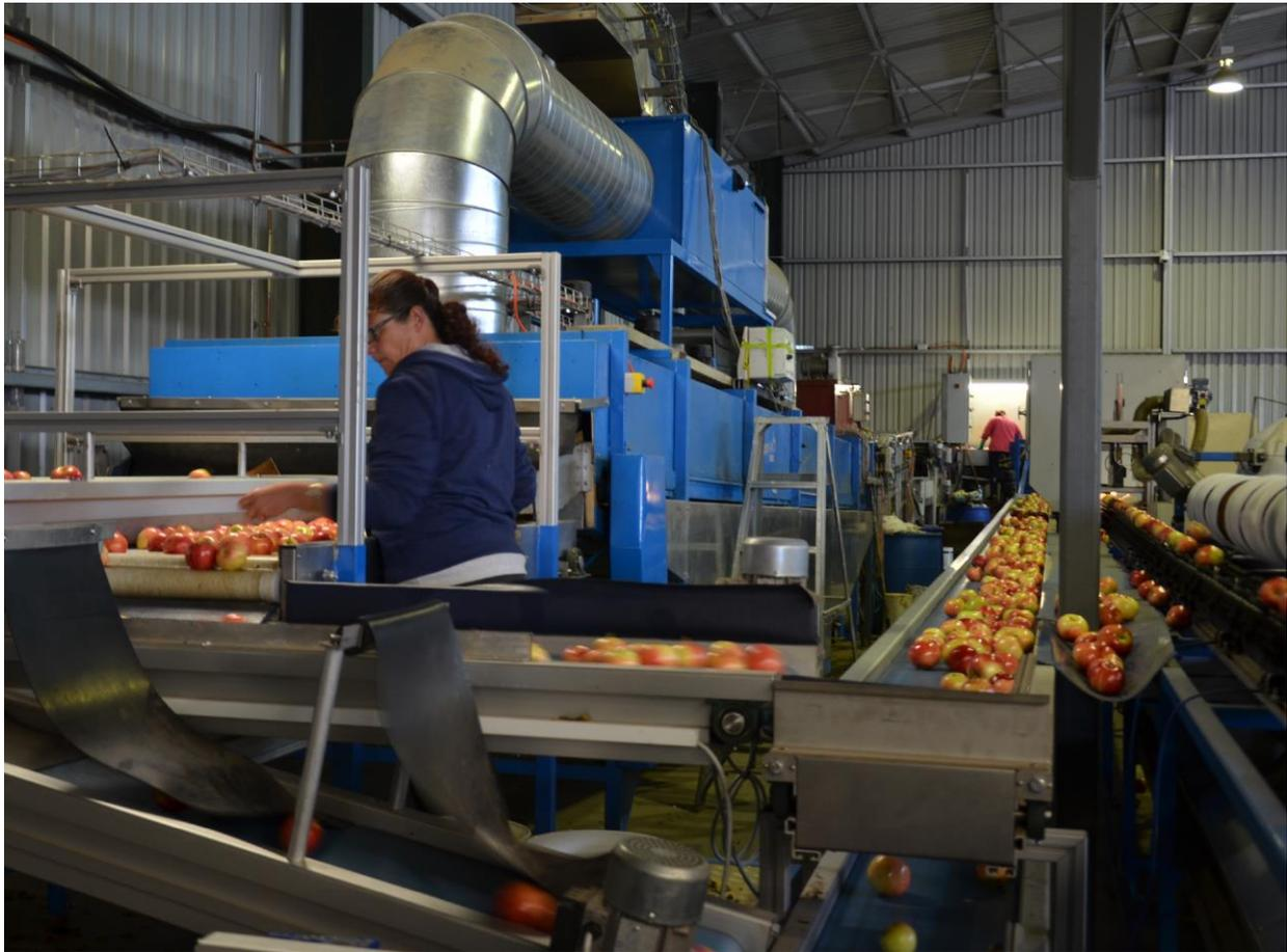
***Advanced drying technologies in apple packing lines can reduce energy costs and ensure apples are perfectly dried.***
