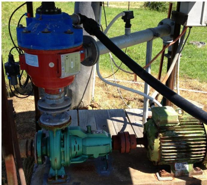
*An older motor that has been left outside and exposed to the elements.*
