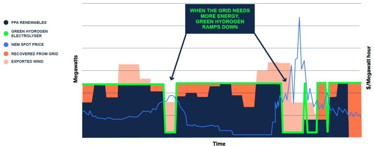
Figure 1 – Active response from electrolyzers supporting reliability and price reductions in the NEM
