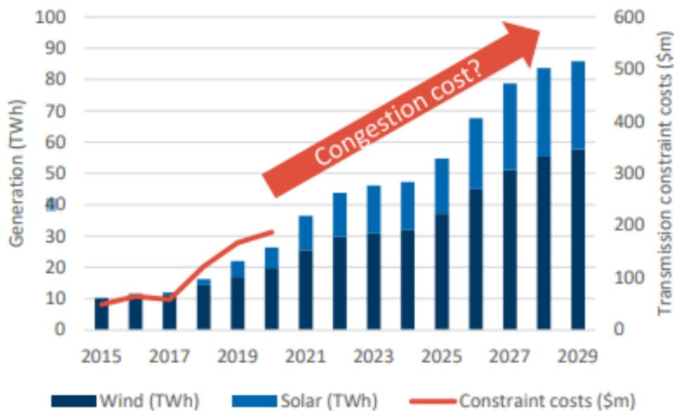
Figure 3 below highlights the problem NSW is facing with congestion; there is already no spare transmission capacity available for renewables. There are currently more than 6,000MW of applications for new renewable generation, but this capacity is unable to be developed until transmission infrastructure is upgraded.
